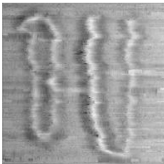
(left) An extremely sharp tungsten wire produced in Lindquist's labs. The tip is only a few 10's to 100's of nanometers wide. (right) A small "BU" etched in a soft gold surface with the tip and then imaged, like a record player, with the same tip. The letters are a few micrometers tall, and the lines are less than 500 nm wide. Images courtesy of Matt Robbins, 2012.
